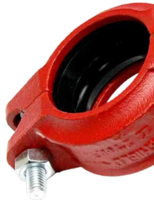
“ SHIELD Rigid Coupling provides rigid joints to prevent liner movement of pipe assembly. With a unique ends locked design, SDG22 coupling can be used when the application or design calls for rigid installations. ”
