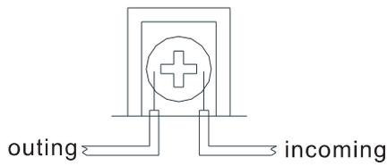
*An uninsulated section of a single conductor should not be looped around the terminal and serve as two separate connections. The wire must be severed, thereby providing supervision of the connection in the event that the wire becomes dislodged from under the terminal.*
